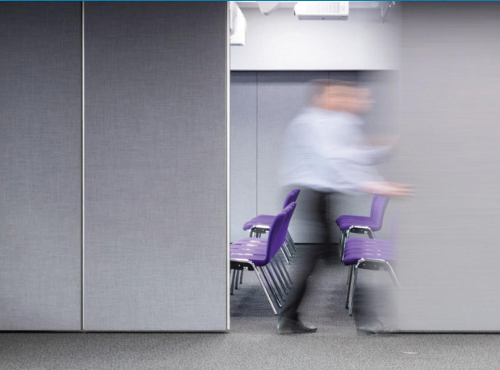
100 is the top of the range and market leader in the world of movable walls. It consists of individually operated top hung panels requiring no floor tracks. Purpose made panels can be manufactured to clients specific requirements, offering total space flexibility, long lasting use and high standards of finishes, sound reduction and durability.
